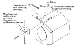
Please Note: If using "S" Hooks, for added safety, crimp both ends of the "S" hooks so the screen cannot come off.
